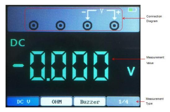
The measuring types include DC voltage (V, mV), AC voltage, DC current (A, mA), AC current (A, mA), resistance, capacitance, diode, and on-off test.
